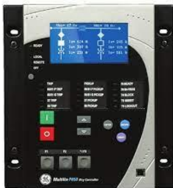
Image-2 GE F650 Bay Controller (used as PU)
